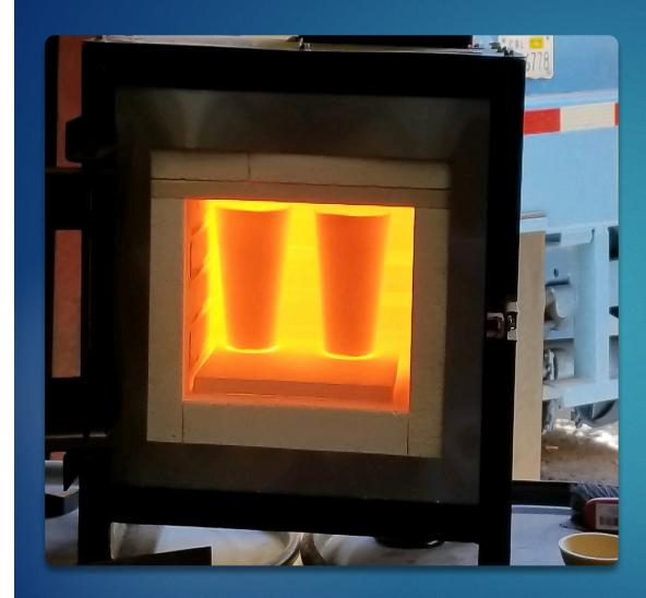
Precious Metals Alloy Being Refined In A Small Assay Furnace
